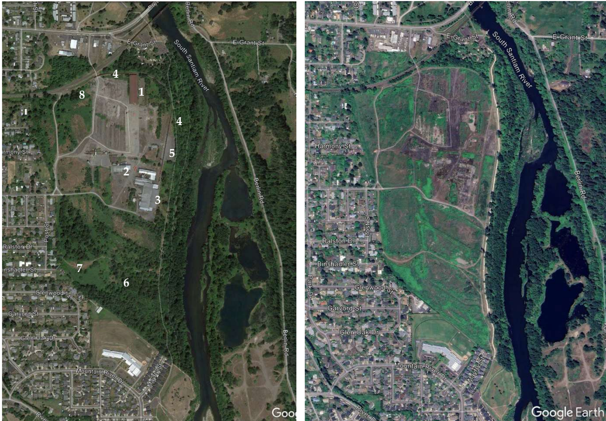
Figure 8. Weyerhaeuser Mill in 2010 (left) and demolished mill site in 2023 (right) (Google Earth 2010, 2023). Buildings and structures visible in 2010, for most the function is inferred: 1) package or finished lumber shed, 2) dry kiln, 3) plywood mill, 4) railway, 5) unknown building, 6) unknown structure, 7) log pond south gate, and 8) log pond north gate.
